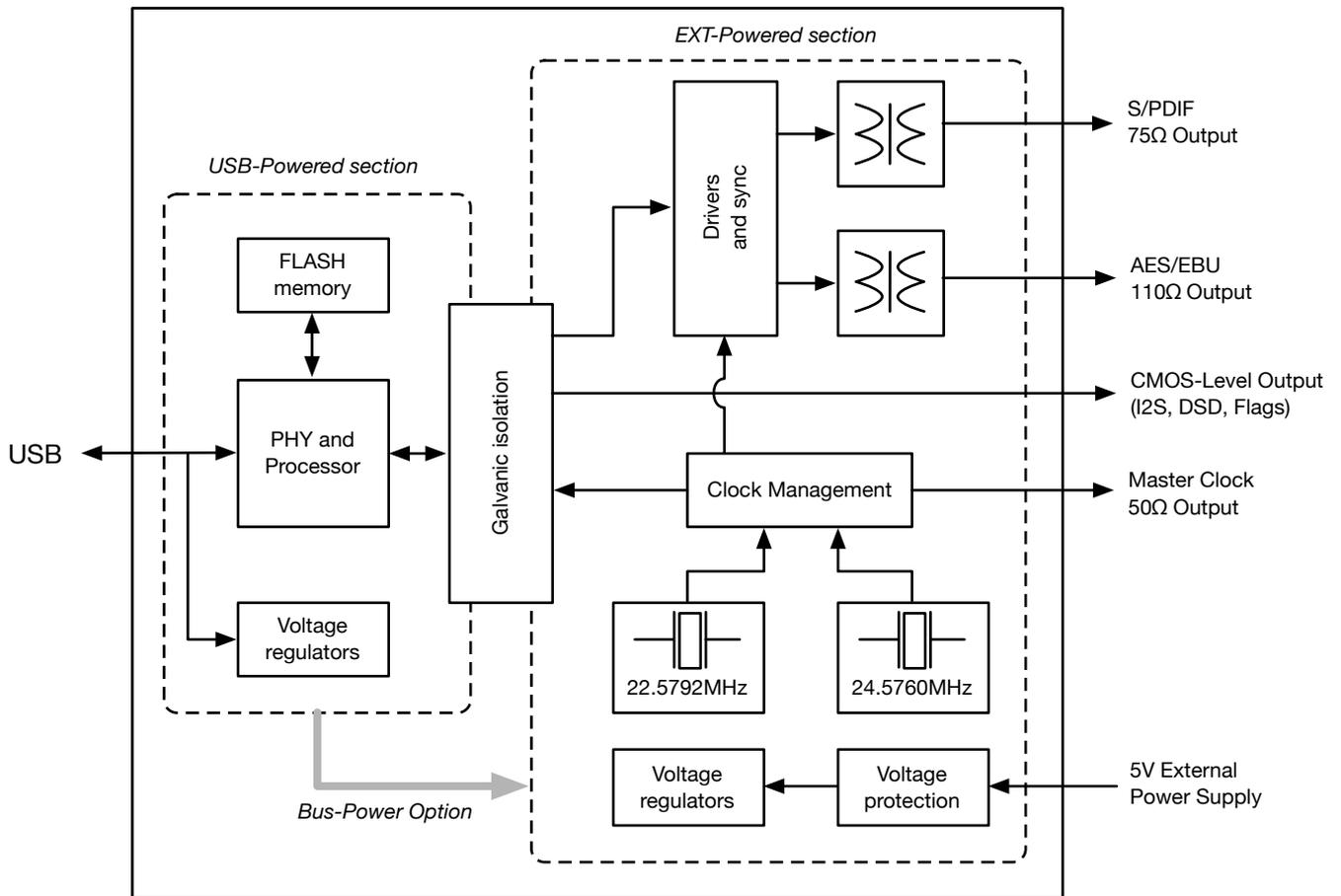
Figure 1-1 – XU2S Functional block diagram
