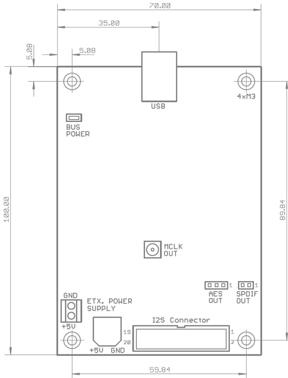
Figure 6-3 – Mechanical dimensions in millimeters
