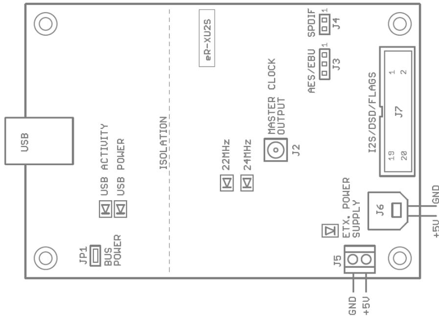
Figure 6-1 – Connectors, LED's and jumpers location
