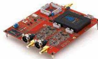
Figure 8: D/A converter reference platform
